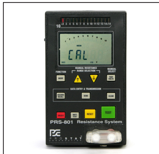
Figure 7: Start the Calibration Sequence by pressing RESET then CLEAR within ½ Second
