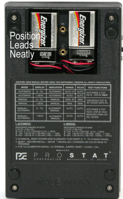
Figure 4: Install 2 each 9V Alkaline Batteries
