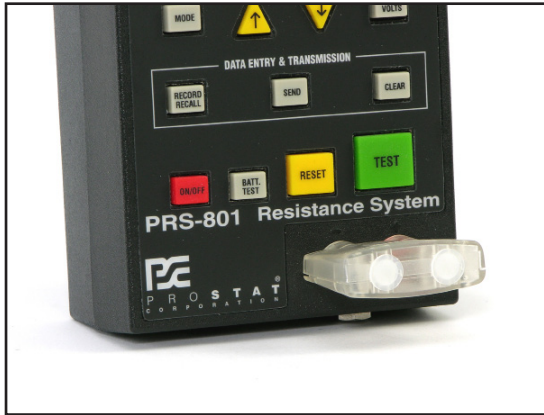
Figure 5: Low Resistance Range Calibration Shunt Installation
