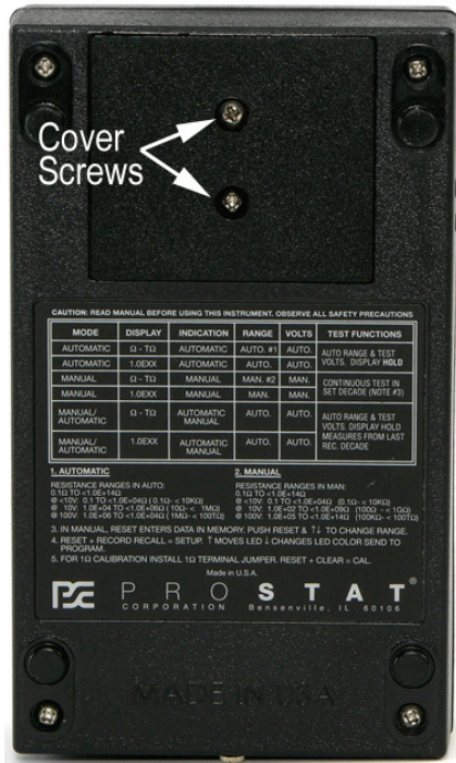
Figure 3: Opening Battery Compartment
