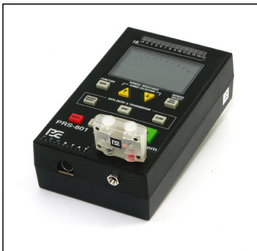
Figure 6: Low Resistance Range Calibration using Reference Module
